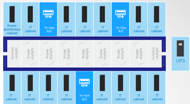
UPS outside of modular data center
